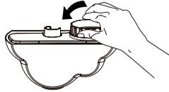
2. Twist the water tank cap counterclockwise to open.
