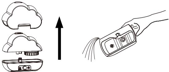
Turn the power OFF and unplug the unit from the electrical outlet. Lift off the outer cover and water tank.
